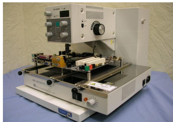
This pre-heater is also designed for use with the SD-3000II to prevent PCB warpage
